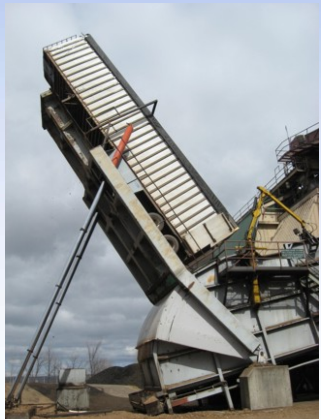
(left to right) Semi trailer parked on a lifting machine. / The hydraulic machine lifts the trailer in the air and the wood is dumped into a holding area. The process takes less than 15 minutes.
