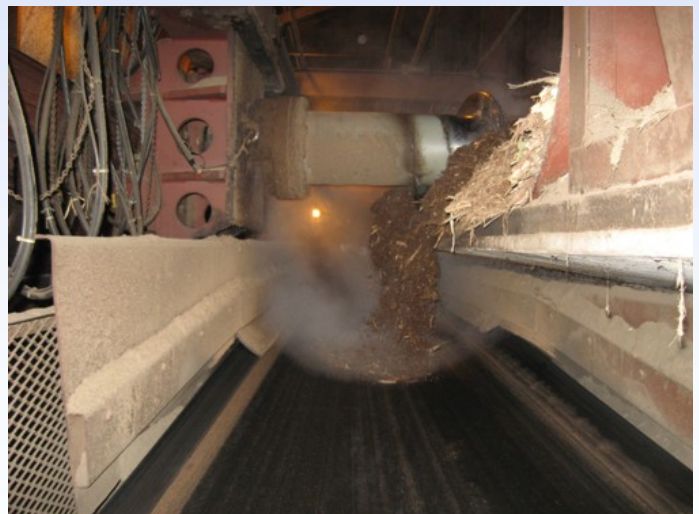
(left to right) A City of Ashland vehicle dumps wood waste. The City of Ashland has the option to dump their wood waste at the Bay Front Plant. / One of two large drills releases wood waste from the enclosed storage container onto the conveyer belt which eventually takes it to the boilers to be burned.
